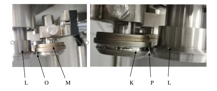
A. Spacing distance between crowner head L and Spin A (spacing distance and
